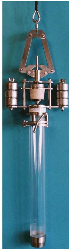
A view of the sediment core sampler
