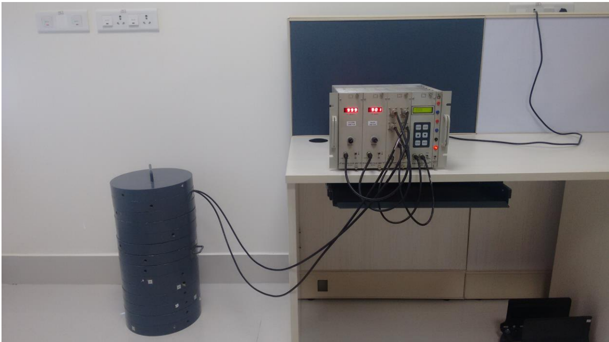
A view of the low background beta counting system
