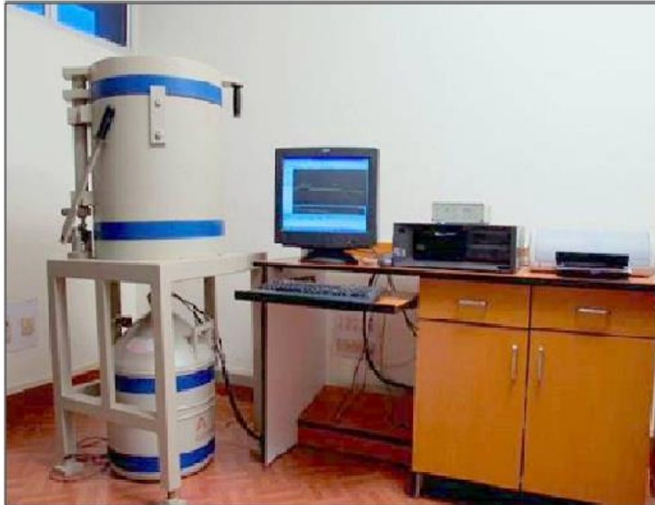
A view of n-type 42% relative efficiency HPGe gamma spectrometer system
