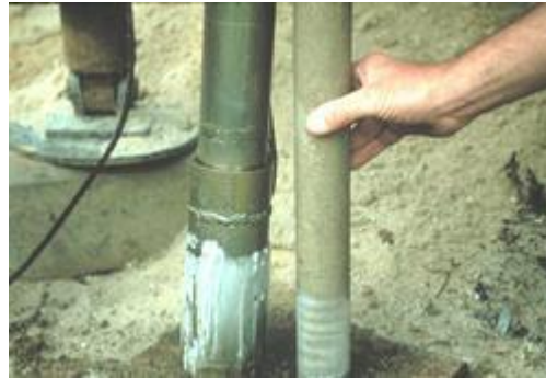
A view of the sediment core sampler
